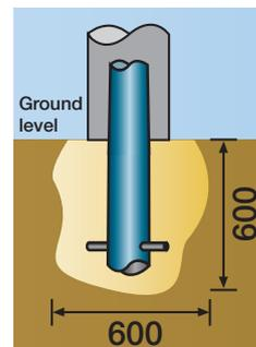
With steel extended root, for setting directly into a concrete foundation.
