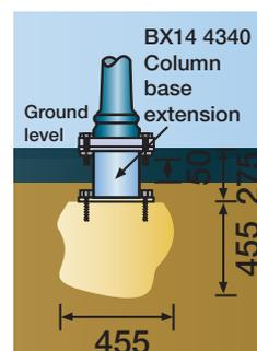
Base extension piece; to allow base plated columns to be secured below ground. Base extension may also be root anchored.
