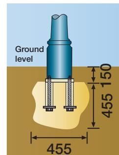
Submerged base plate for bolting to concrete block below ground level.
