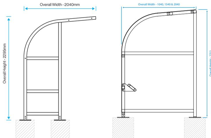
Vertically Clad Diagram
