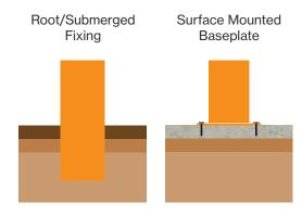
Standard Unit Dimensions: Length: 1830mm Width: 470mm Height: 440mm Root Length: 300mm Weight: 30kg
