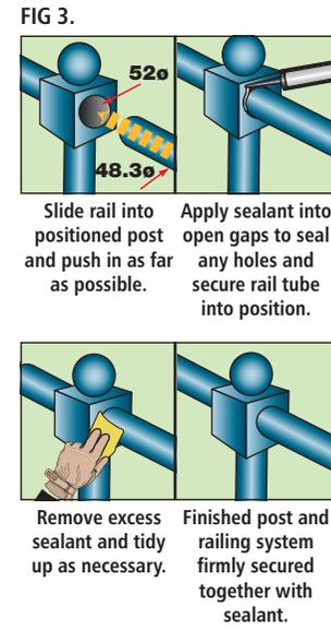
Rail tube is secured into the rail posts using a betafil 1025 polyurethane sealant as indicated in FIG 3. Tube of sealant £7.50. Sealant gun £4.90.
