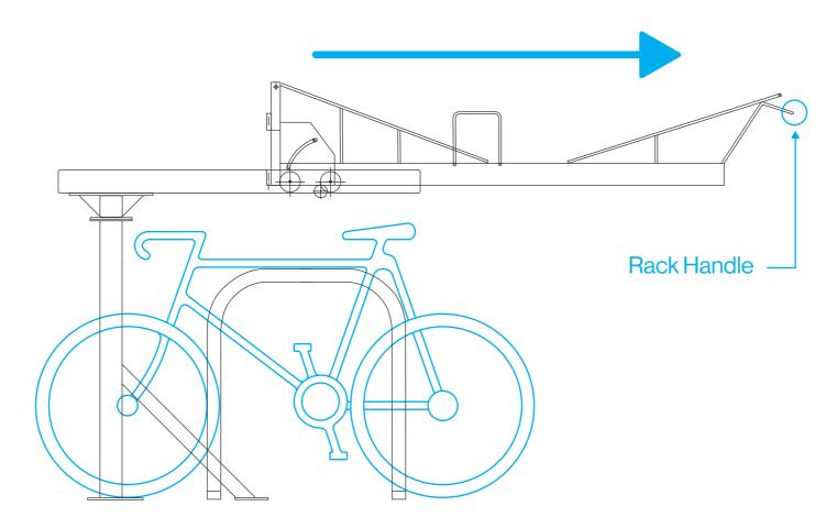
When releasing the cycle rack you must take the handle and lift slightly, Thenstart to carefully pull cycle rack towards you.
