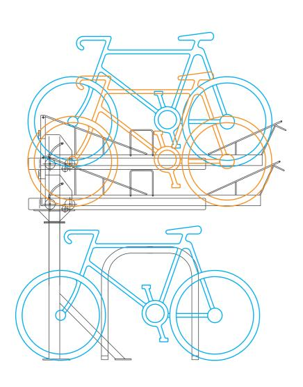
The Diagram above shows an Easi-Riser Two-Tier Cycle Rack in full use.
